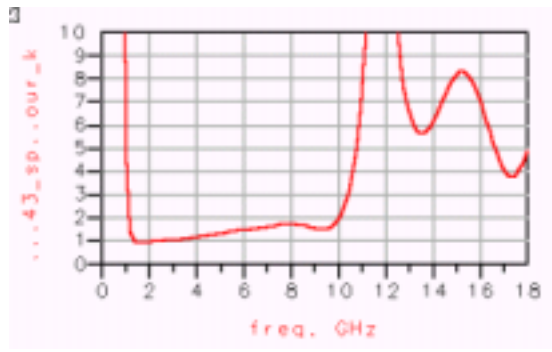
Figure 15. HP ADS Simulation showing Stability Factor K
