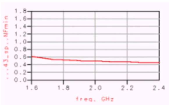
Figure 14 HP ADS Simulation showing Noise Figure
