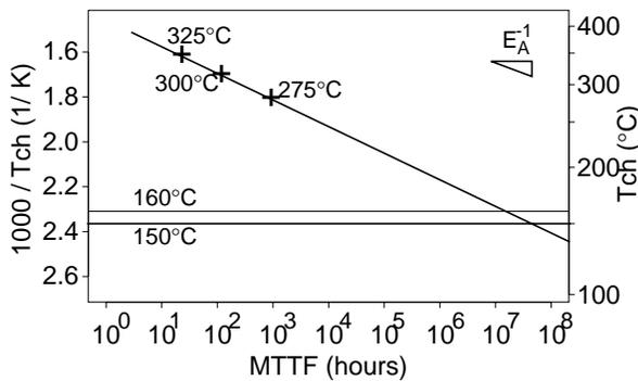
**Figure 3. Arrhenius Plot for  $I_{DSS}$**
