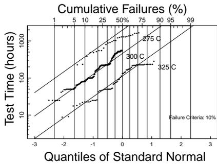
**Figure 2. Log-Normal Distribution of  $G_M$  Drift Failures**
