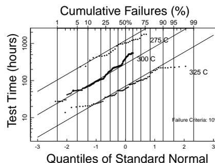
**Figure 1. Log-Normal Distribution of I<sub>DSS</sub> Drift Failures**
