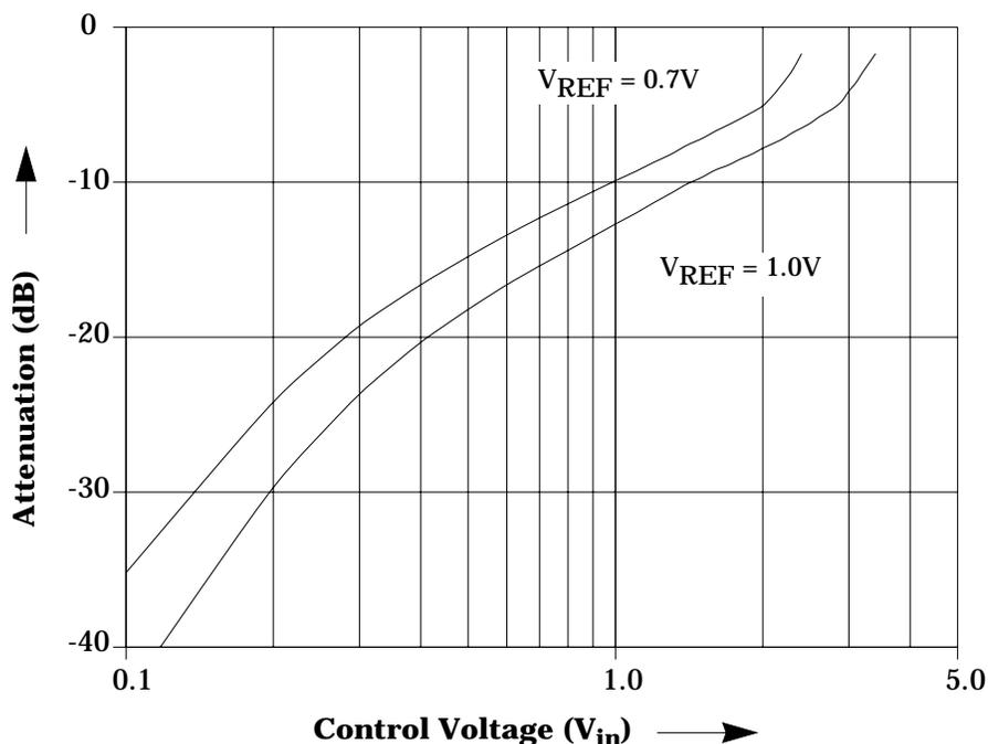
**Figure 3. HMMC-1002 Attenuation vs. Control Voltage ( $V_{in}$ ) @ 13.0 GHz**
