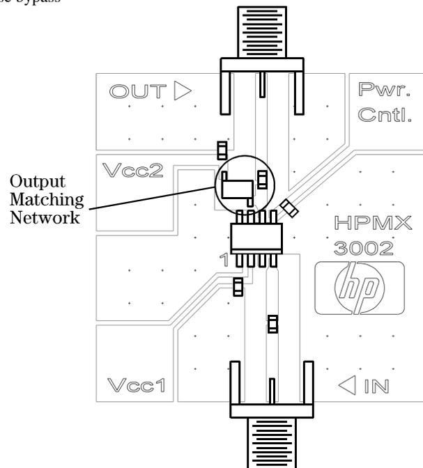
Figure 1. Assembled HPMX-3002 demonstration circuit board
