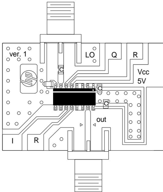
Figure 1. Assembled board showing HPMX-2003 with bypass and blocking capacitors.
