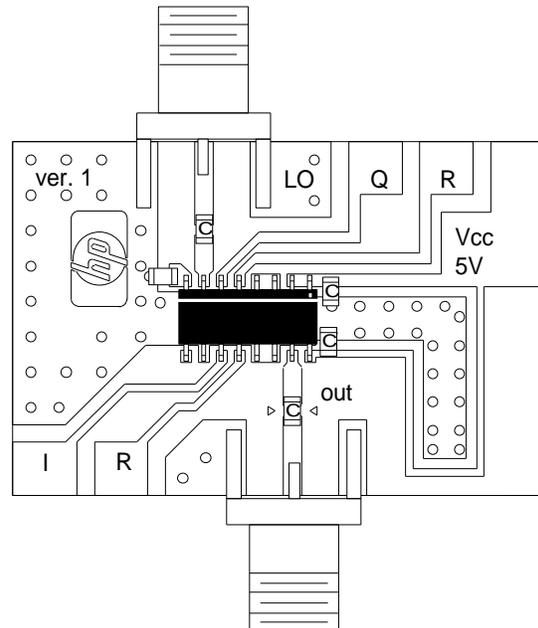
Figure 2. Assembled board showing HPMX-2005 with bypass and blocking capacitors.
