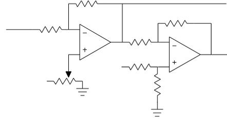
Figure 4. DC bias circuit for I and Q inputs (balanced drive)
