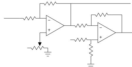
Figure 4. DC bias circuit for I and Q inputs
