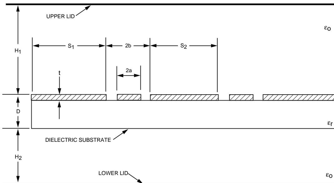
Figure 15. CoPlanar Waveguide with Top and Bottom Covers.
