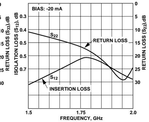
Figure 13. Transmitter Arm Insertion Loss.
