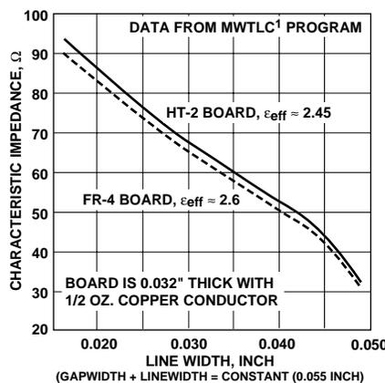
Figure 5. Impedance vs. Linewidth, CoPlanar Waveguide.
