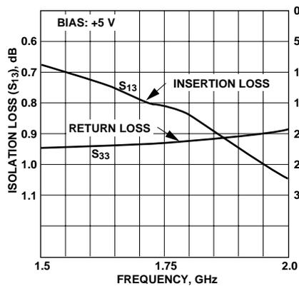
Figure 12. Receiver Arm Insertion Loss.
