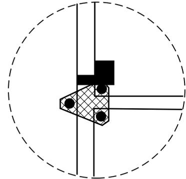
DETAIL SHOWING TRIANGULAR CONNECTING PATCH ON UNDERSIDE.
