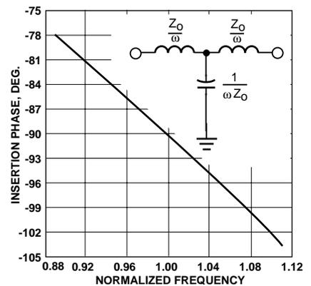
Figure 6. 90° Phase Delay Circuit.
