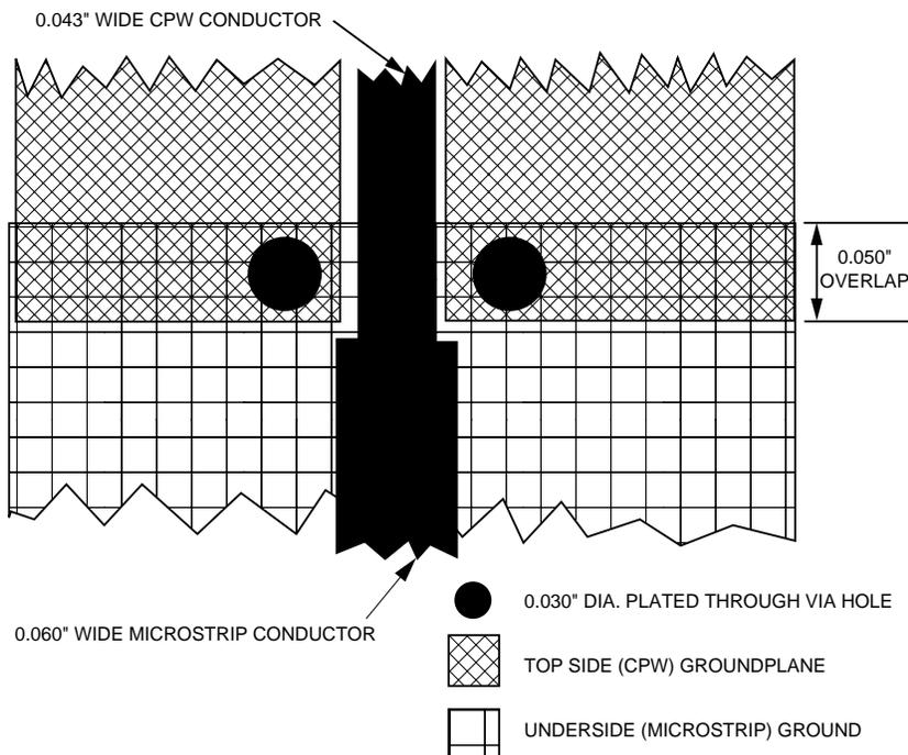
Figure 9. Microstrip to CPW Transition on 0.032" HT-2.
