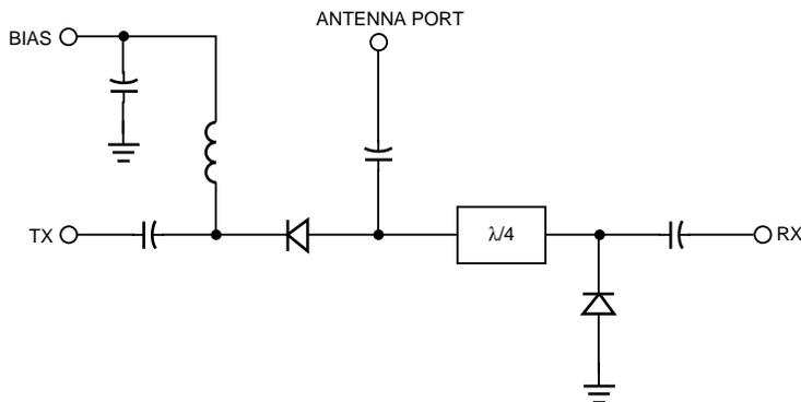
Figure 1. Low Current T/R Switch.
