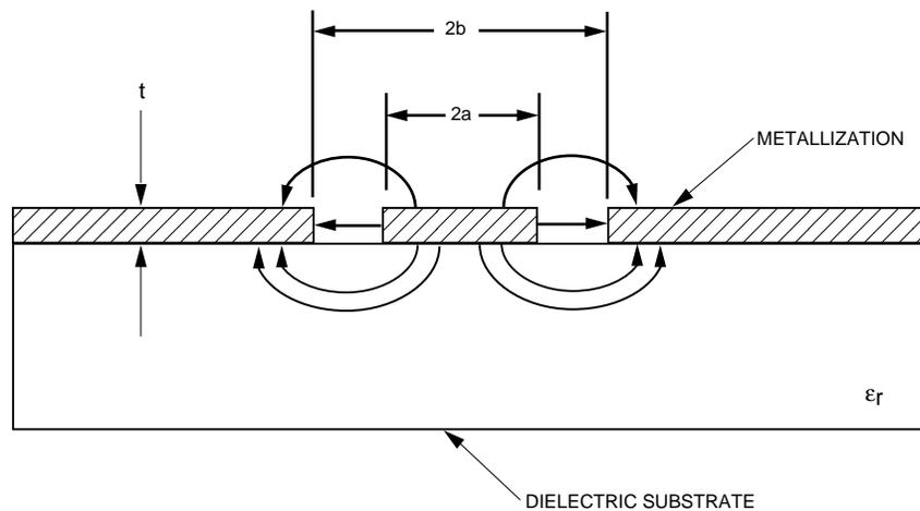
Figure 14. Cross-Section of CoPlanar Waveguide.
