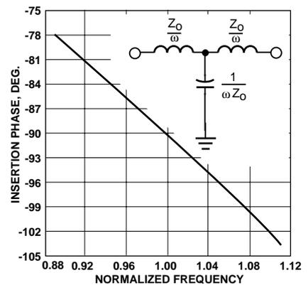
Figure 6. 90° Phase Delay Circuit.
