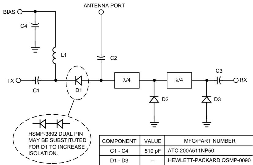
Figure 7. Schematic of the prototype Switch.
