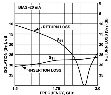
Figure 10. Receiver Arm Isolation.
