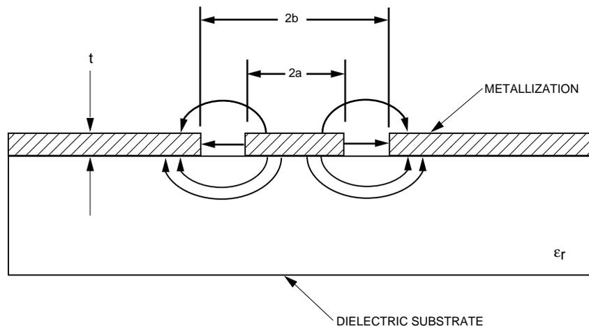
Figure 14. Cross-Section of CoPlanar Waveguide.
