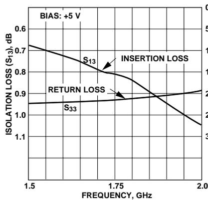
Figure 12. Receiver Arm Insertion Loss.
