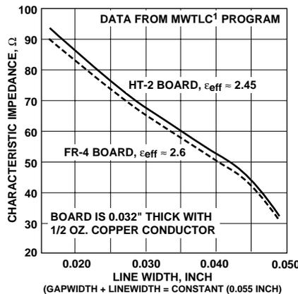
Figure 5. Impedance vs. Linewidth, CoPlanar Waveguide.
