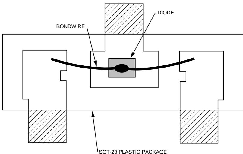
Figure 3. HSMP-4890 Low Inductance Diode.
