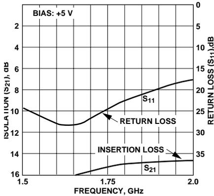
Figure 11. Transmitter Arm Isolation.
