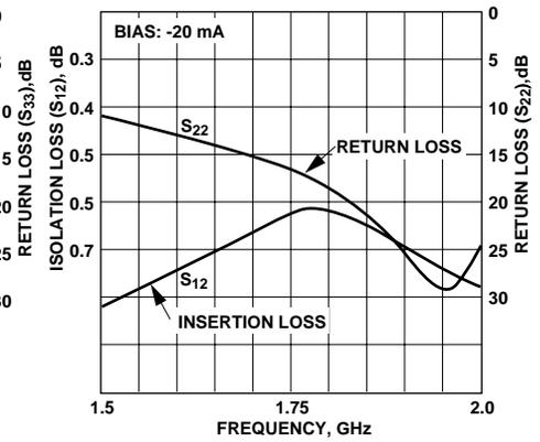
Figure 13. Transmitter Arm Insertion Loss.
