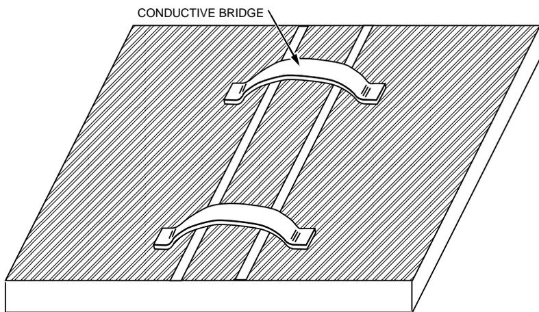
Figure 16. CPW with Conductive Bridge.
